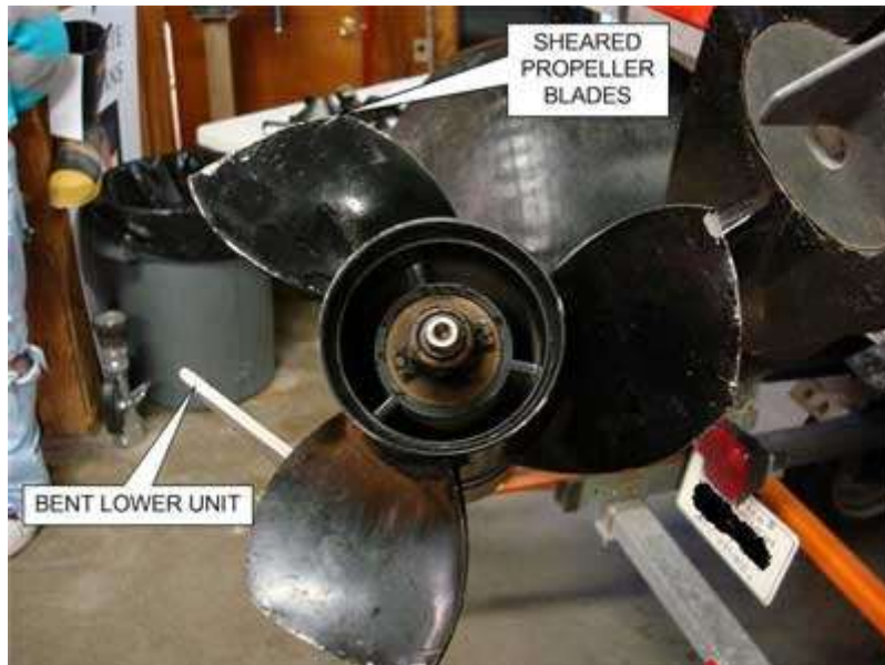
Photo 1. Picture of damaged lower unit and propeller. (NIOSH photo.)
